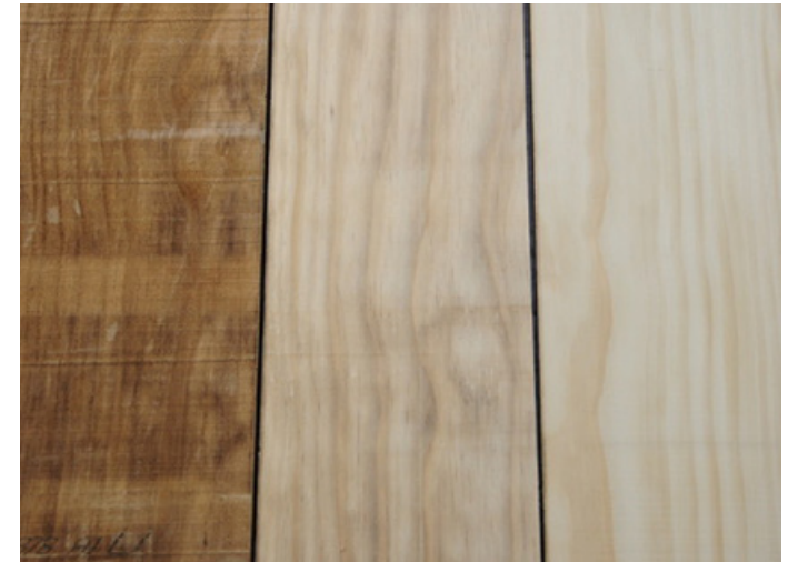
DISCOLOURATION: ROUGH BOARD, AFTER SURFACING 3MM AND AFTER SURFACING 6MM FROM ROUGH
